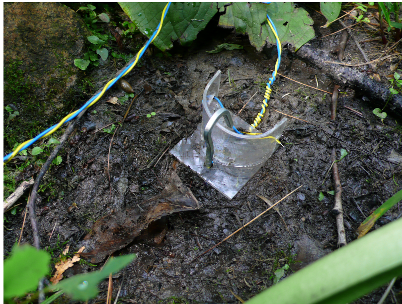
Figure 1: Electronic resistance (ER) sensor schematic.
