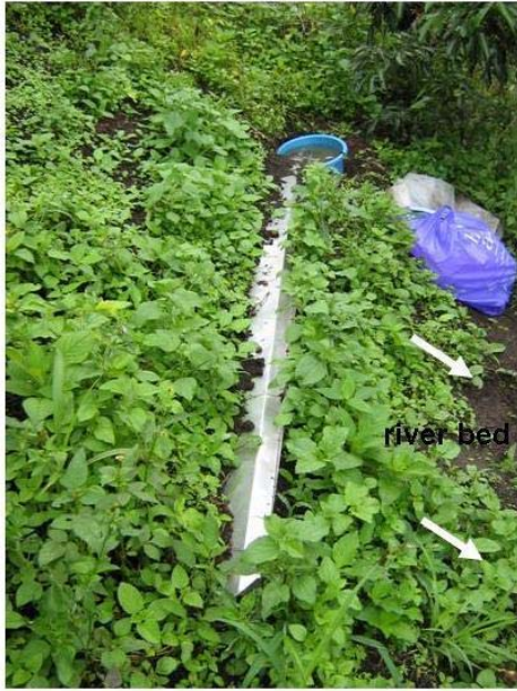
Figure A3: The trench (metal sheet) which was used to collect surface runoff. The picture was taken after a storm event 2007, before the bucket was emptied. The bucket is covered during events to avoid dilution by direct rainfall and is cleaned from substrate, whenever it is emptied.
