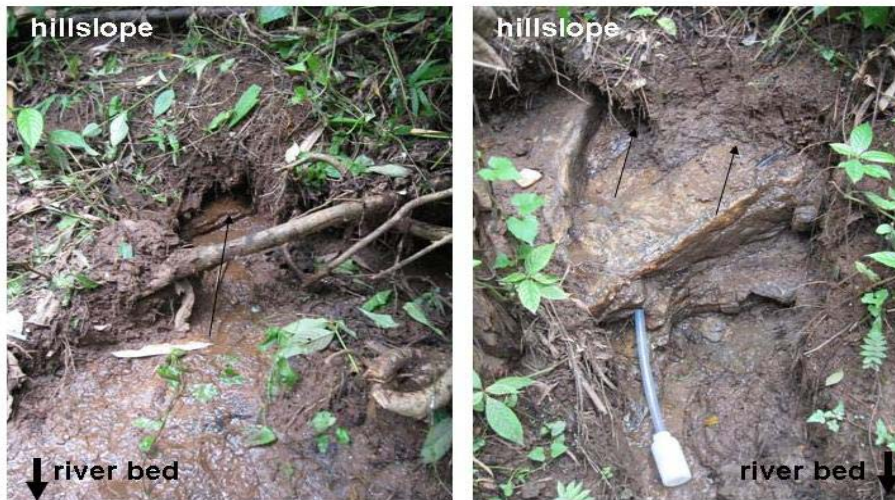
Figure A2: Leakage of soil water at the foot hill in 2009. The arrows indicate the line of leakage between the soil cover and bed rock close to the river bed along the foot slope. The right picture shows the sampling bottle, while water was collected.
