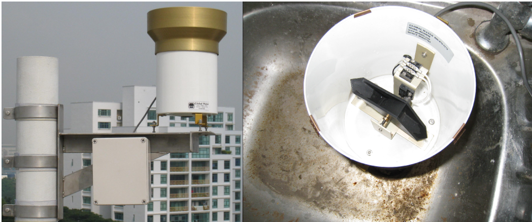
Fig. 1. Rainfall measurement setup.
