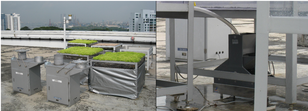
Fig. 2. Runoff measurement setup.
