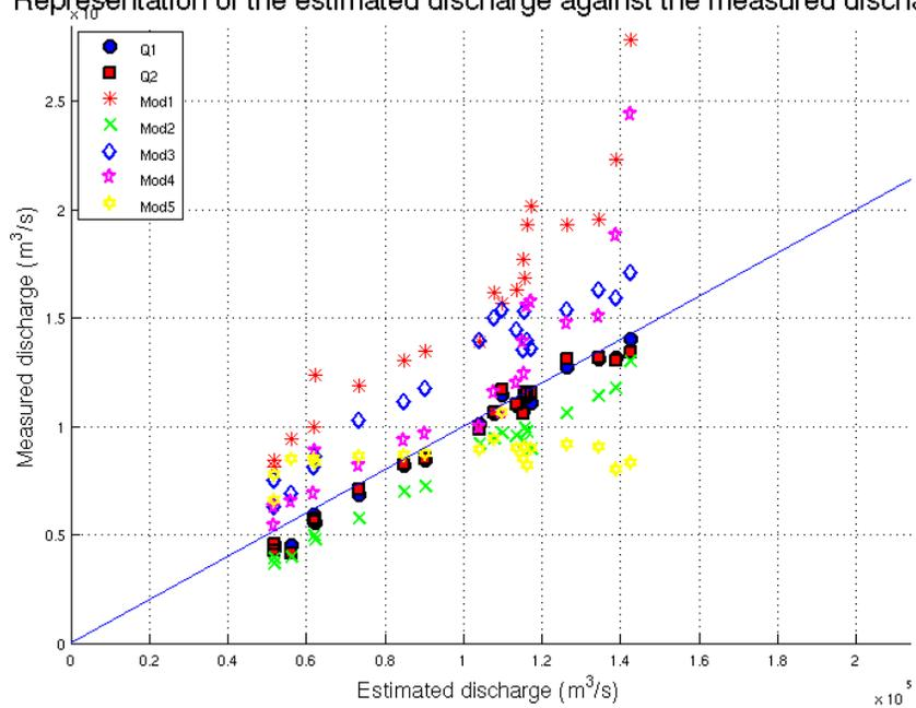
**Fig. 4.** Representation of the estimated discharge against ADCP discharge measurements on Manacapuru dataset.
