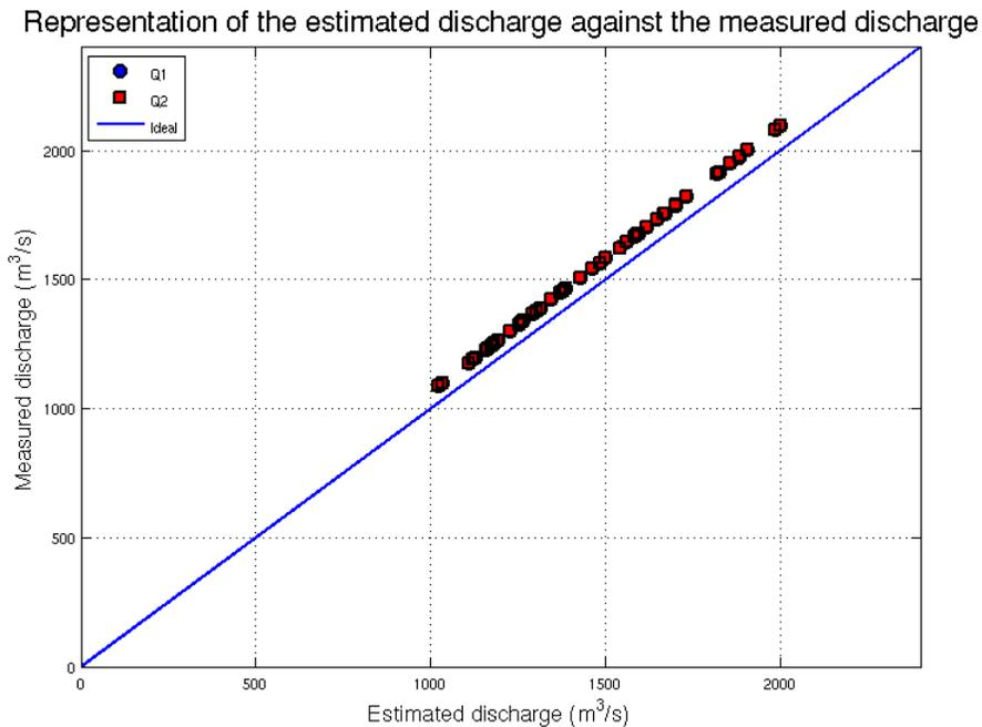
**Fig. 3.** Representation of the estimated discharge using Eqs. (8) and (9) against simulated discharge measurements.
