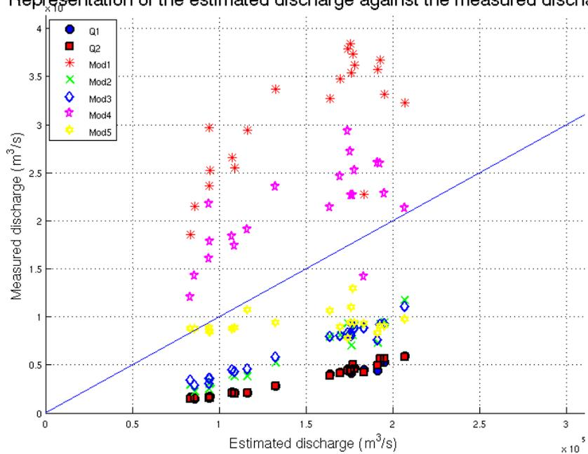
**Fig. 5.** Representation of the estimated discharge against ADCP discharge measurements on Obidos dataset.
