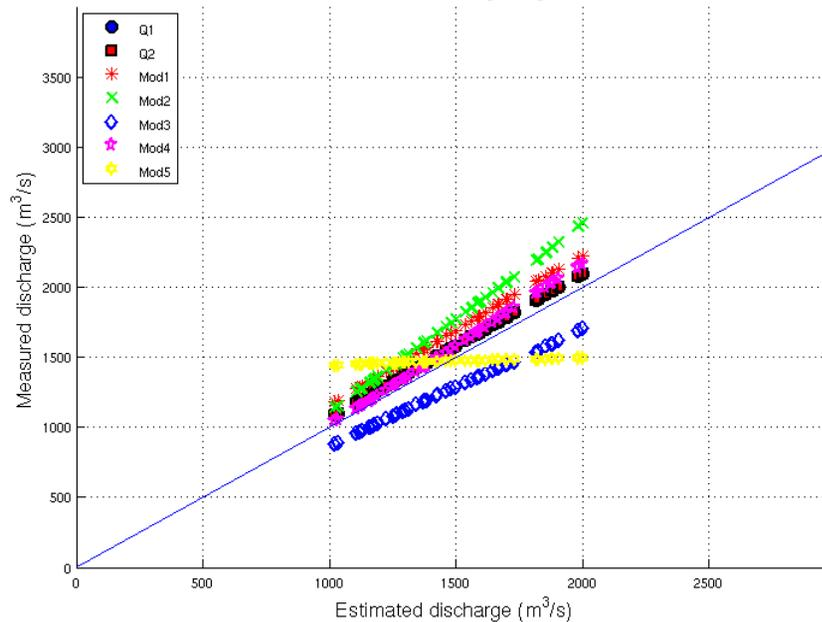
**Fig. 6.** Representation of the estimated discharge against simulated discharge measurements.
