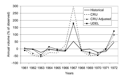
**Fig. 5.** Deviations (%) from observed of simulated mean annual flow volumes of the Okavango River at Rundu (using the main calibration period of 1961 to 1972) based on different input rainfall data. "Historical" data are based on local gauges.
