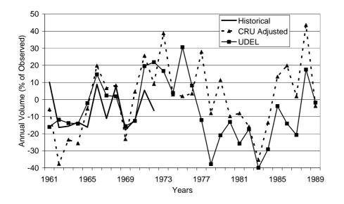
**Fig. 6.** Deviations (%) from observed of simulated mean annual flow volumes of the Okavango River at Mukwe (using the whole baseline period of 1961 to 1990) based on different input rainfall data. "Historical" data are interpolated local gauges, described in Wilk et al., 2006.
