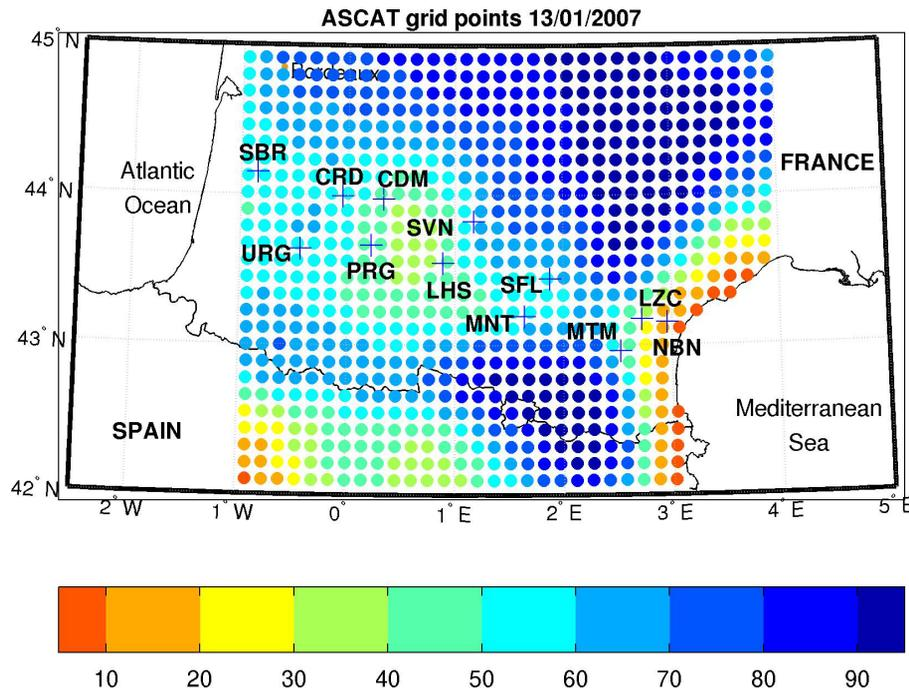
**Fig. 2.** ASCAT SSM product (in units of %) over Southwestern France for 13 January 2007. Data are issued by EUMETSAT and resampled to the Discrete Global Grid (DGG, 12.5 km grid spacing) of TU-Wien (Institute of Photogrammetry and Remote Sensing, Vienna University of Technology). Blue crosses denote the twelve stations of the SMOSMANIA network.
