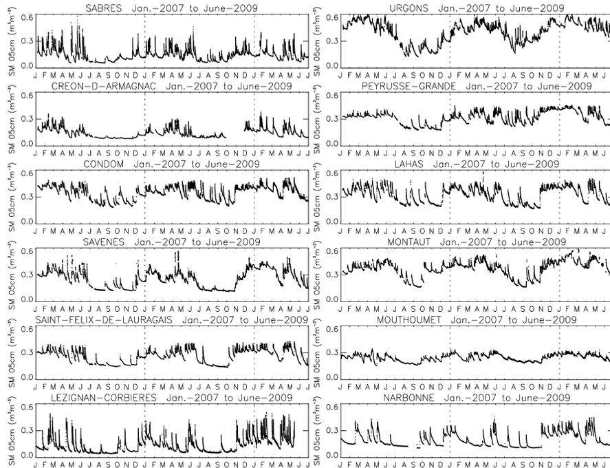
**Fig. 1.** Daily average 5 cm (SSM) volumetric soil moisture content ( $\text{m}^3 \text{m}^{-3}$ ) for the twelve stations of the SMOSMANIA network over a two year and six month period (January 2007–June 2009)
