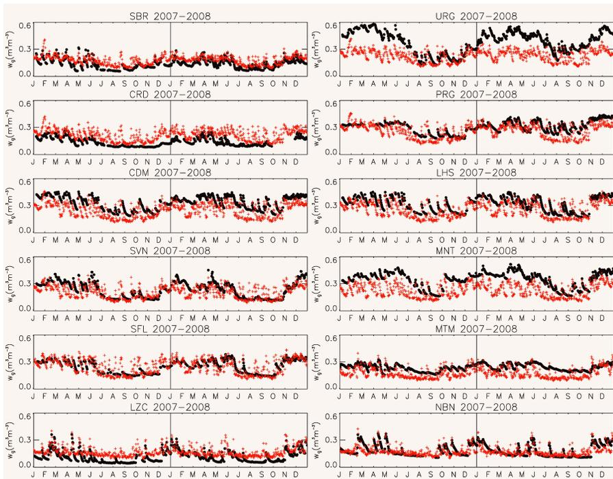
**Fig. 3.** Comparison between synthetic SSM from the SIM model (red crosses) and in situ SSM (black dots) for the twelve stations of the SMOSMANIA network over a two year period (2007–2008).
