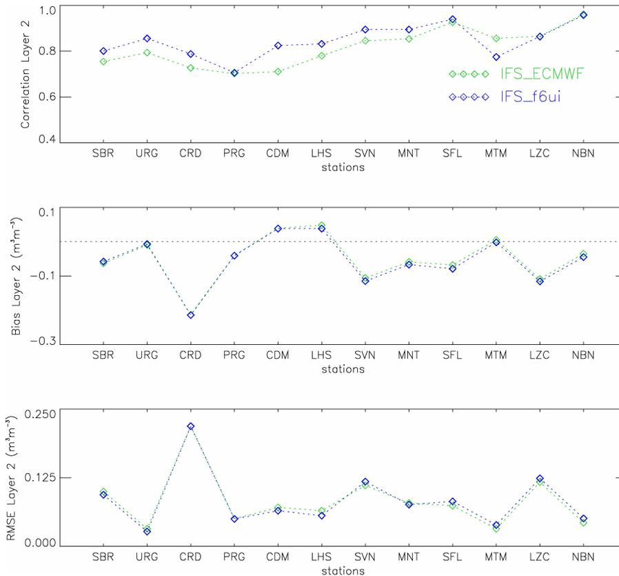
**Fig. 9.** Evaluation of the ECMWF root-zone (7–21 cm) soil moisture analysis using the soil moisture observations at 20 cm of the twelve stations of the SMOSMANIA network. From top to bottom: correlation, mean bias and RMSE.
