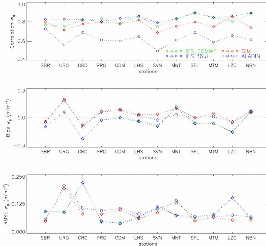
**Fig. 8.** Score of the Météo-France and ECMWF SSM analyses using the twelve stations of the SMOSMANIA network. From top to bottom: correlation, mean bias and RMSE. In situ SSM observations are used to evaluate SSM analysis from Météo-France (ALADIN in blue dots and SIM in red diamonds) and ECMWF (Optimal Interpolation with  $T_{2m}$  and  $RH_{2m}$  in green diamonds, SEKF with  $T_{2m}$  and  $RH_{2m}$  and ASCAT SSM estimates in blue diamonds).
