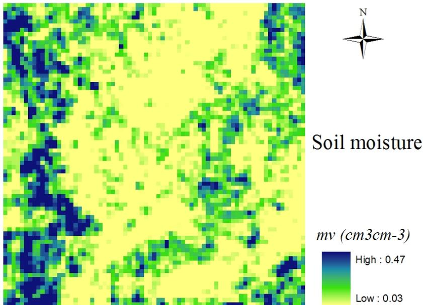
**Fig. 6.** Retrieved mv in the study area based on the results of the surface roughness acquired by the proposed multi-angular algorithm.
