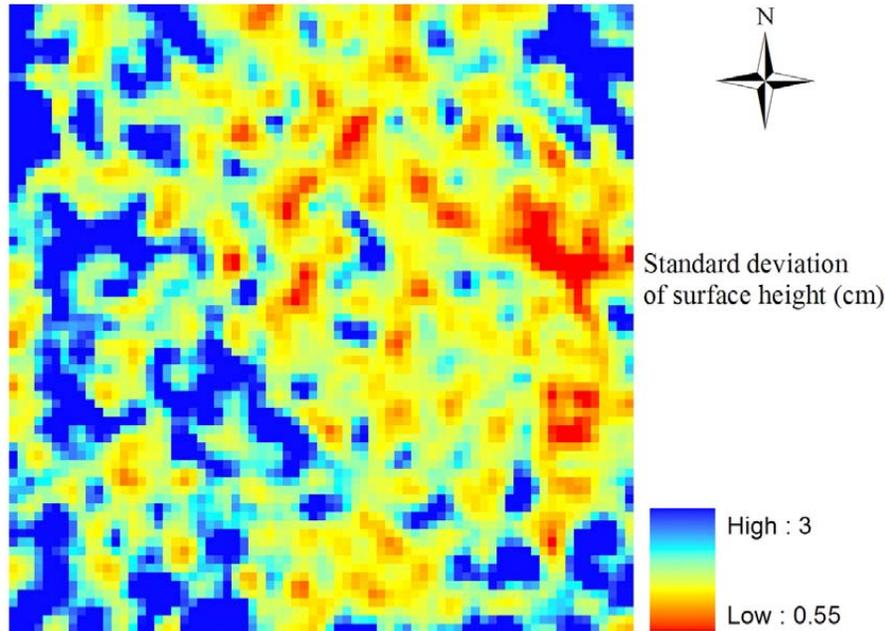
**Fig. 5.** Estimated result of standard deviation of surface height based on two images with swath modes of *IS1* and *IS7* in association with Eqs. (9)–(13).
