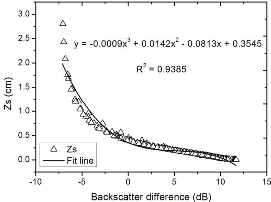
Fig. 4. Sketch map of the relationship between  $Z_s$  and  $\Delta\sigma_{IS1-IS7}$  (incidence angles of  $18.5^\circ$  and  $43.9^\circ$ ) provided by Eq. (11).
