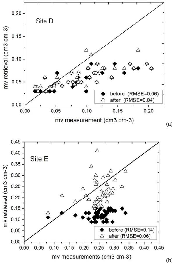
**Fig. 7.** Comparison between mv estimated from radar imagery and from in situ measurements at (a) site D and (b) site E before vegetation correction (before,  $\blacklozenge$ ) and after elimination of the canopy effect (after,  $\triangle$ ).
