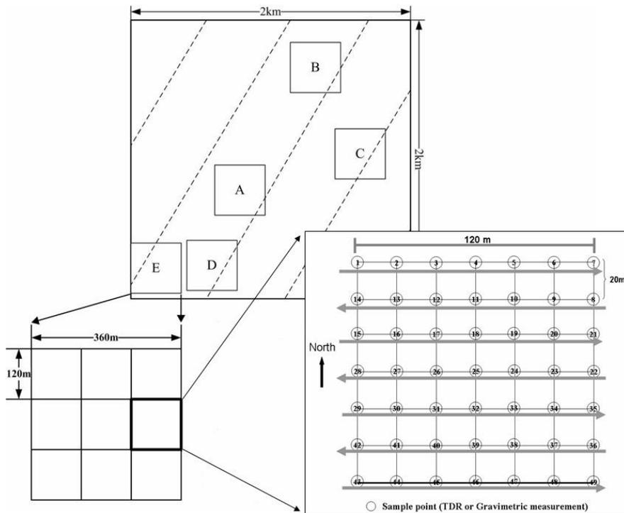
**Fig. 2.** The three-level soil moisture sampling strategy designed for use in field campaigns. Resolution ranges from coarse to fine, corresponding to the foci experimental area, experimental site, and elementary sampling plot.
