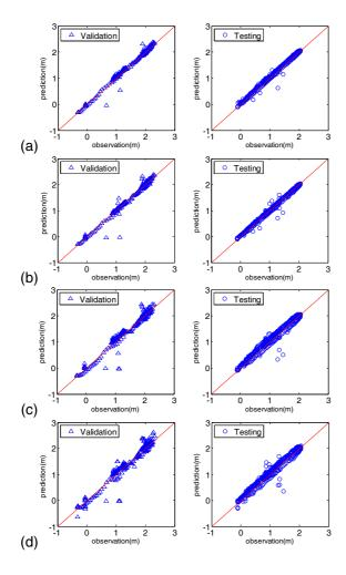
Fig. 6. The scattering plots of the RNN outputs versus the observations for (a) 5-, (b) 10-, (c) 15-, and (d) 20-min-ahead predictions in both validation and testing sets.
