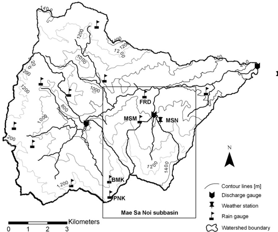
**Fig. 1.** Mae Sa watershed and Mae Sa Noi sub-catchment with measurement devices (FRD, MSM, MSN, BMK and PNK are representative rain gauges for the sub-catchment Mae Sa Noi).
