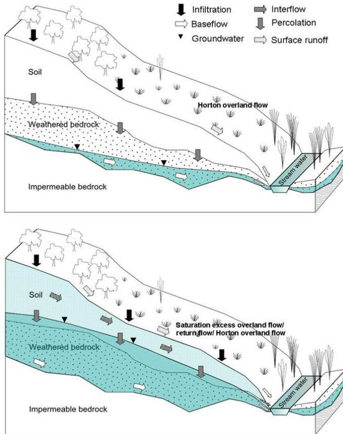
Fig. 10. Conceptual model of runoff generation at Mae Sa Noi hillslope during saturated and unsaturated conditions.
