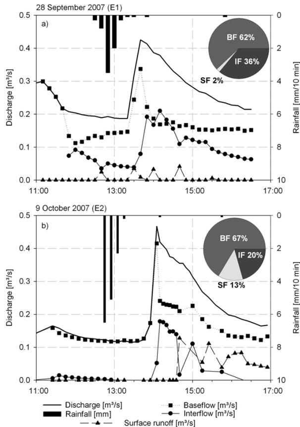
**Fig. 9.** Three component hydrograph separation for E1 (September 2007) and E2 (October 2007) showing fractions of baseflow (BF), interflow (IF) and surface runoff (SF) based on silica concentration and EC measurement.
