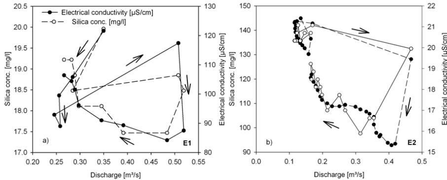
**Fig. 6.** Silica concentration and electrical conductivity during (a) 28 September 2007 (E1) and (b) 9 October 2007 (E2). Arrows indicate the course of time.
