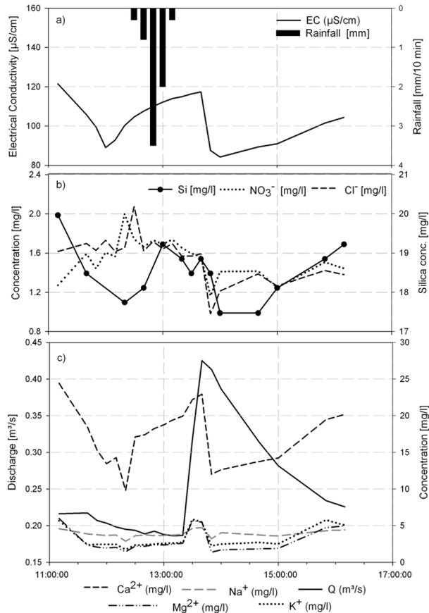
Fig. 3. Event on 28 September 2007 (E1) showing EC values, silica and ion concentrations, discharge and rainfall.
