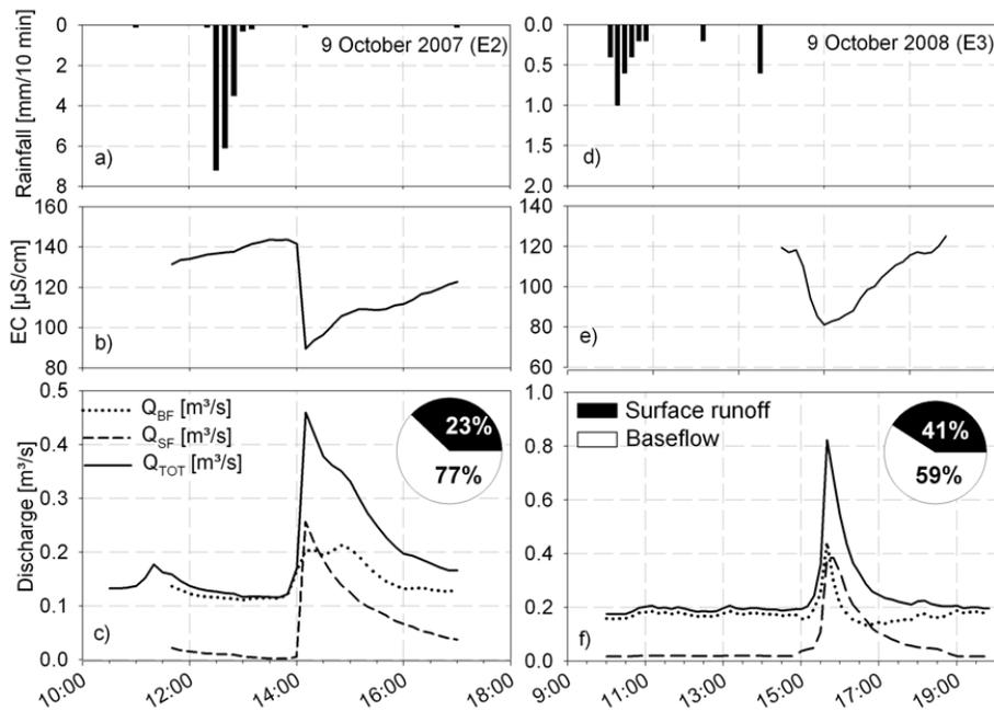
**Fig. 8.** Results of the two-component hydrograph separation for 9 October 2007 (E2) and 9 October 2008 (E3) based on surface runoff measurements. ( $Q_{TOT}$ : total discharge;  $Q_{SF}$ : surface runoff component,  $Q_{BF}$ : baseflow component).
