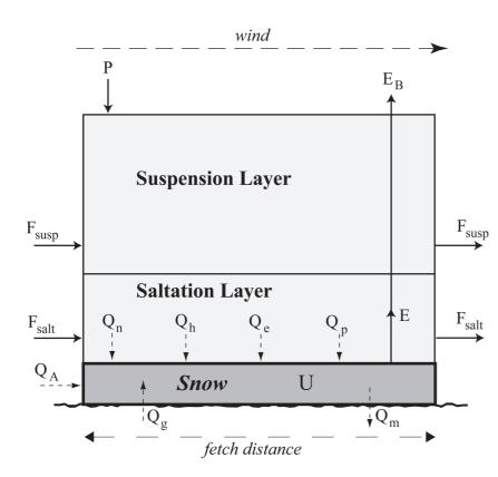
Fig. 3. Control volume for blowing snow mass fluxes and snowmelt energy.
