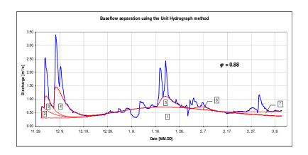
Fig. 1. Baseflow separation using the unit hydrograph method (Su, 1995).
