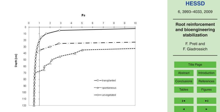
**Fig. 11.** Factor of safety (*Fs*) versus depth in unvegetated soil, transplanted stand or natural slope under the following conditions: saturated bulk unit weight [kN/m<sup>3</sup>],  $\gamma_{sat} = 20 \text{ kN m}^{-3}$ , water unit weight  $\gamma_w = 9.8 \text{ kN m}^{-3}$ , slope angle  $\beta = 26.5^{\circ}$ , soil friction angle  $\phi' = 20^{\circ}$ , soil cohesion = 1 kPa, surcharge  $W_v = 0-0.196-0.4$  kPa, respectively. Cv(z) as in Fig. 10. All plants are about seven years old.
