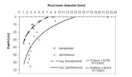
Fig. 6. Root mean diameter versus depth of transplanted and spontaneous Spanish Broom plants.
