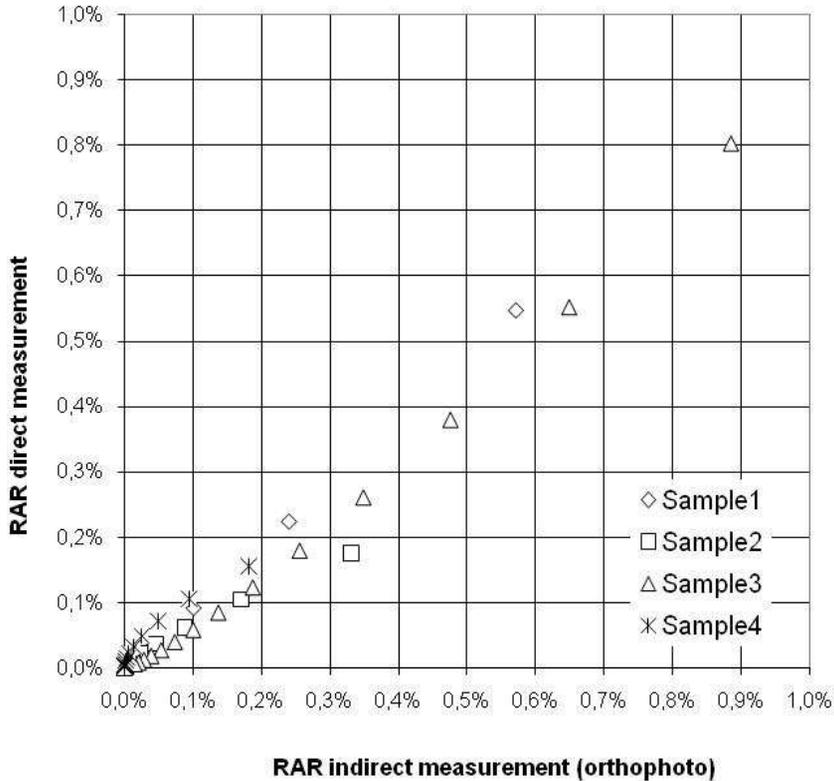
**Fig. 4.** RAR estimation (four Spanish Broom *specimens*) using the direct and indirect method.
