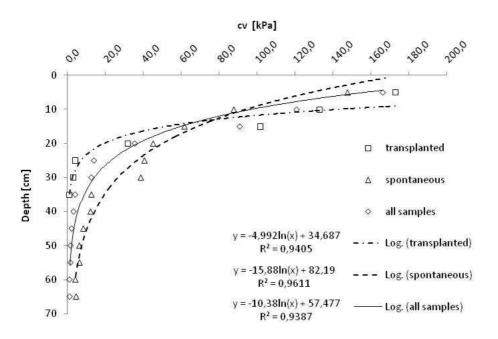
**Fig. 10.** Root cohesion Cv versus depth of transplanted, spontaneous and all Spanish Broom plants: the first line represents the plants transplanted in the study area (Gentilino); the second line represents the plants growing spontaneously in the neighboring area (Gabbiola and Spedaletto); the continuous line refers to all samples.
