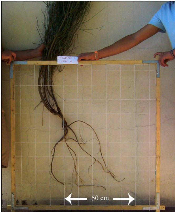
**Fig. 2.** Specimen of naturally grown Spanish Broom (square grid size 10 cm).
