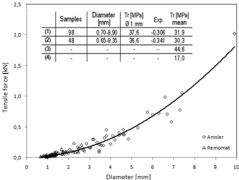
**Fig. 9.** Tensile force [kN]  $tr$  versus root diameter of Spanish Broom. The line shows the second order polynomial regression curves fitted to the experimental data:  $tr = 0.0203 d^2 + 0.0062 d$   $R^2 = 0.94$ . The regression equation of tensile strength [MPa]  $Tr$  versus root diameter [mm] of Spanish Broom curve is (1)  $Tr = 37.605 d^{-0.306}$   $R^2 = 0.29$ . Comparison between literature data: (2) Tosi (2007); (3) Laranci et al. (2004); (4) Norris and Greenwood (2003).
