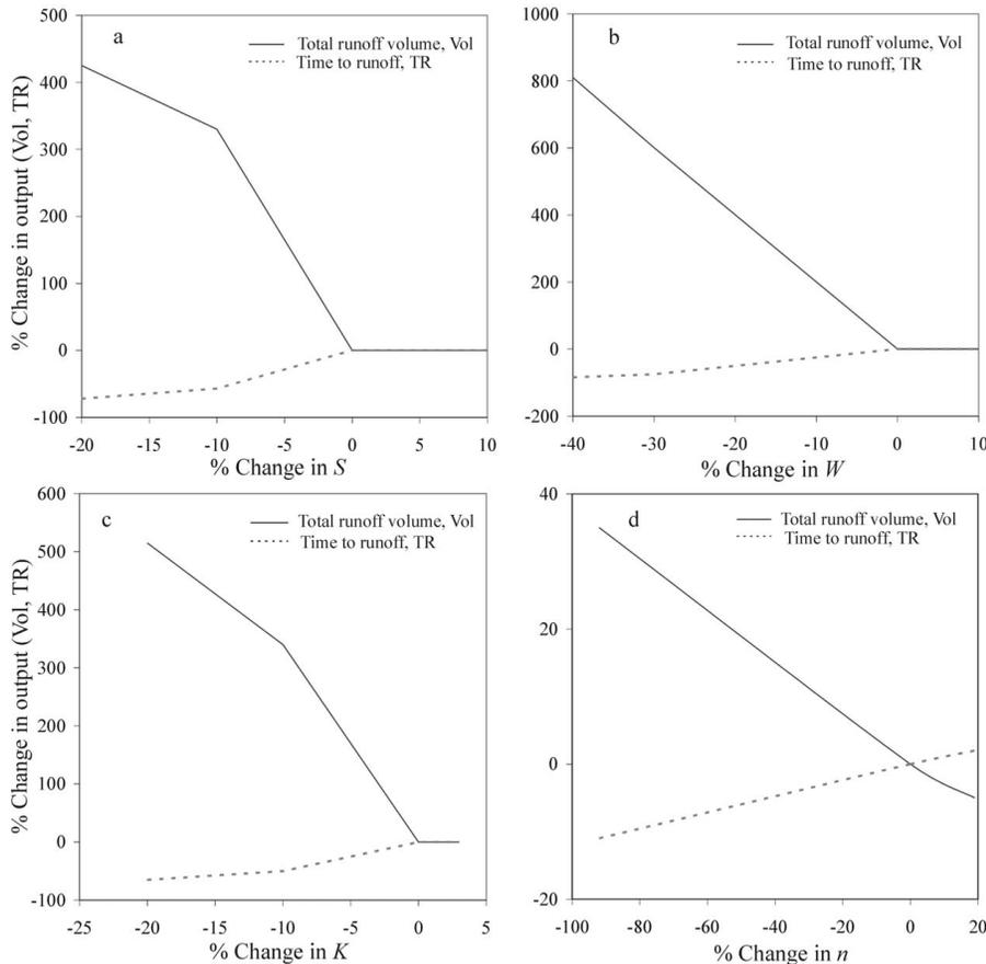
**Fig. 6.** Sensitivity of the model to changes in the input values of the sorptivity, runoff width, hydraulic conductivity and Manning’s roughness coefficient.
