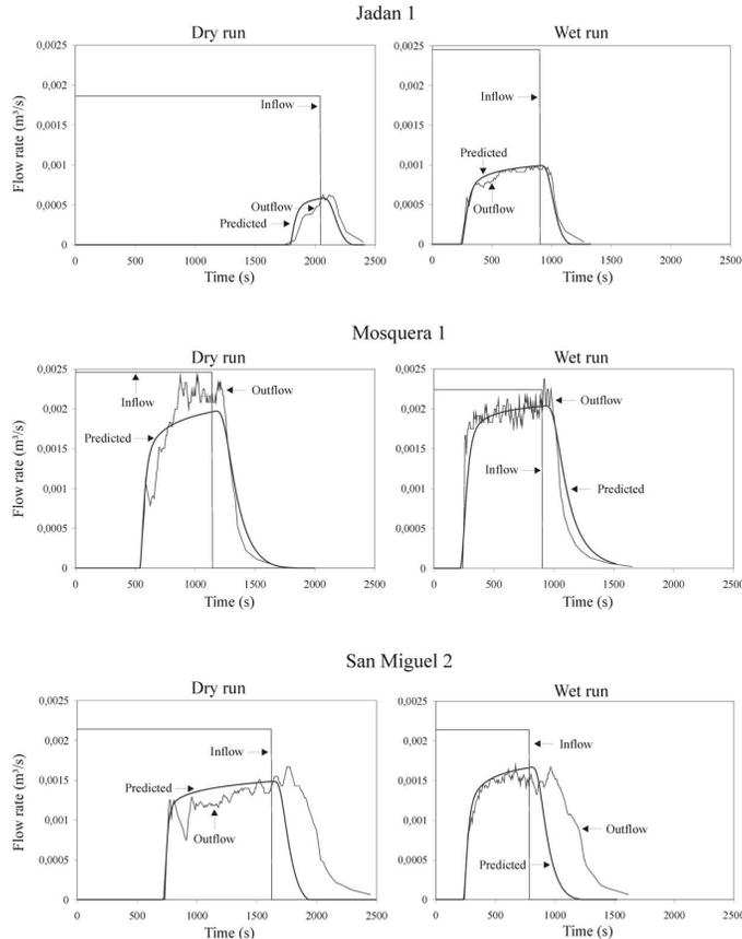
**Fig. 4.** Observed and computed flow hydrograph for three gullies with distinct vegetation cover of the gully bed (Jadan1: dense vegetation cover, Mosquera1: intermediate vegetation cover, and San Miguel2: very low vegetation cover of gully bed).
