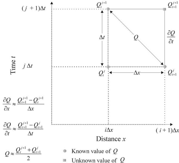
**Fig. 3.** Outline of the computational grid used to solve the kinematic wave equation (after Chow et al., 1988).
