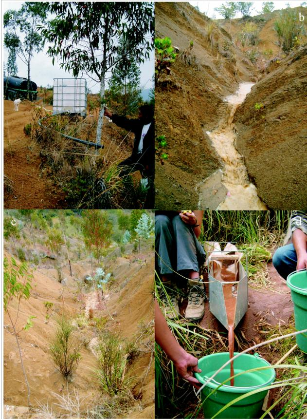
**Fig. 1.** Experimental design of the concentrated flow experiments with **(a)** water supply from water tank, **(b)** and **(c)** concentrated flow in the gully floor, and **(d)** collection of runoff water and sediment.
