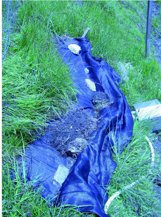
Fig. 4. Soil erosion during the vegetation period 2007. Large pieces of soil were collected in the sediment traps ranging from 1 to 30 cm.
