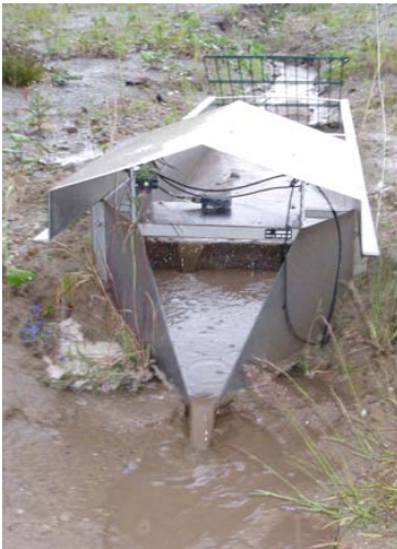
Fig. 9. Flume and registration of surface runoff during a rainstorm (maximum rain intensity 8.5 mm/10 min; 25 June 2008).
