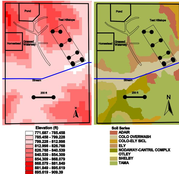
**Fig. 4.** (A) Digital Elevation Map of the test field. (B) IPSAID soils map for the test field. The test field is denoted by a box. Transects where field samples were collected are denoted by the black line with circles.
