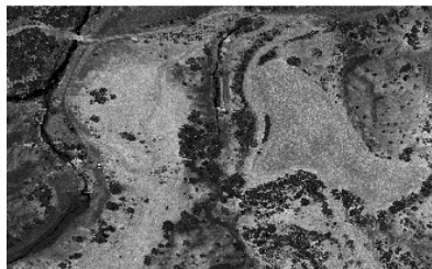
(c) Corrected return intensity of the first echo from the laser fluctuations. Values are represented in grey level scale and stretched between 0 and 150.
