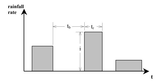
Fig. 1. The rectangular pulse model of precipitation.
