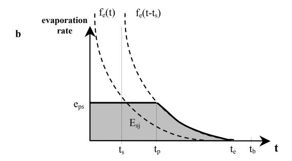
Fig. 3. The dynamics of: (a) infiltration, and (b) evaporation from the soil surface.
