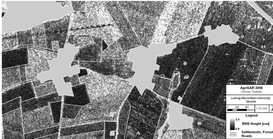
Fig. 7. Derived RMS Heights from the relation between the Re_{[\rho_{RRLL}]} and the in-field soil surface roughness.
