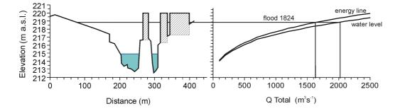
**Fig. 3.** Cross profile A5 from Stuttgart (Neckar River) with the stage-discharge curve and energy line (standard Manning's *n*) during the highest stage of the 1824 flood.
