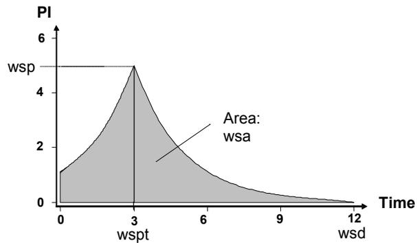
**Fig. 2.** Double exponential function for internal rainfall structure.
