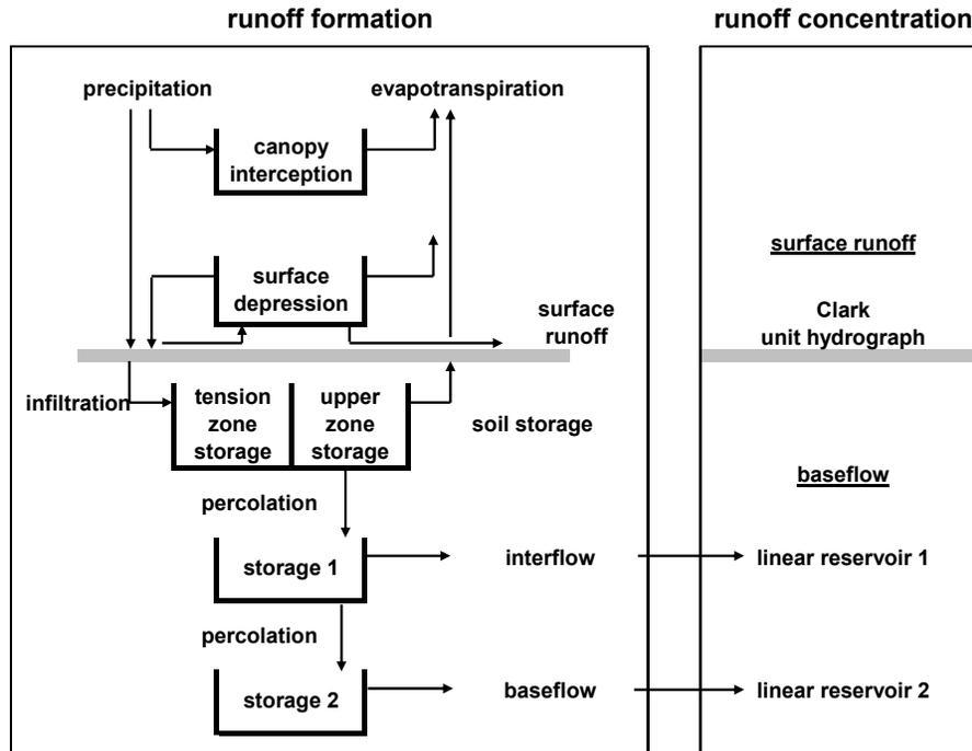
Fig. 4. Selected structure of the hydrological model HEC-HMS.
