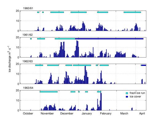
**Fig. 3.** Calculated ice discharge at Gauging Station 30 at Krokur. River discharge is taken same as in Fig. 2, 200 m<sup>3</sup> s<sup>-1</sup>. Horizontal bars indicate days with ice observed. Light blue bars indicate slush or frazil ice runs. Dark blue bars indicate ice cover.
