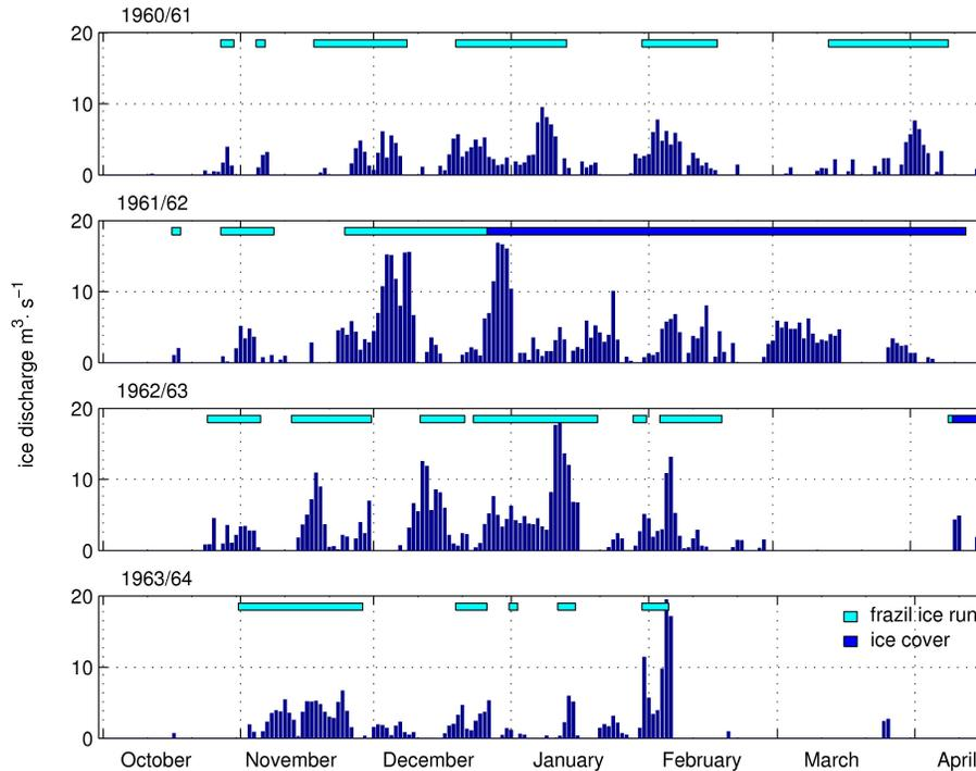
**Fig. 3.** Calculated ice discharge at Gauging Station 30 at Krokur. River discharge is taken same as in Fig. 2,  $200 \text{ m}^3 \text{ s}^{-1}$ . Horizontal bars indicate days with ice observed. Light blue bars indicate slush or frazil ice runs. Dark blue bars indicate ice cover.
