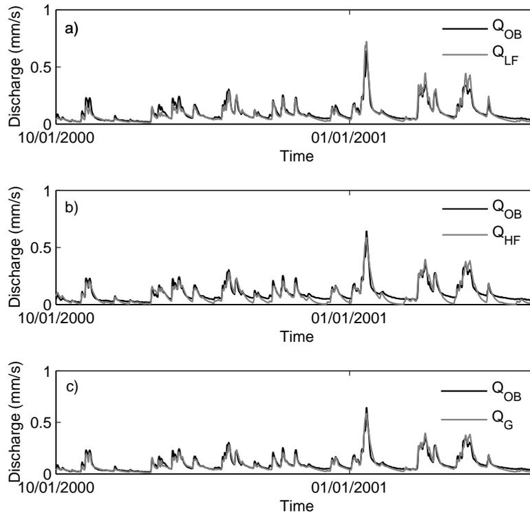
**Fig. 5.** Hydrograph comparison **(a)** low-flow model; **(b)** high-flow model; **(c)** model combination (Eq. 12).
