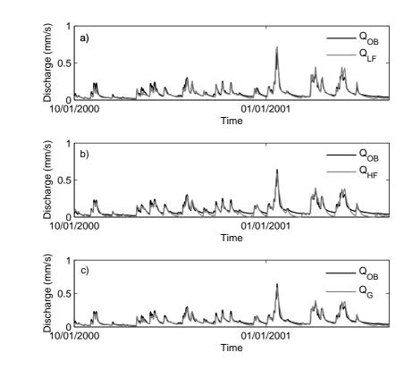
**Fig. 5.** Hydrograph comparison **(a)** low-flow model; **(b)** high-flow model; **(c)** model combination (Eq. 12).
