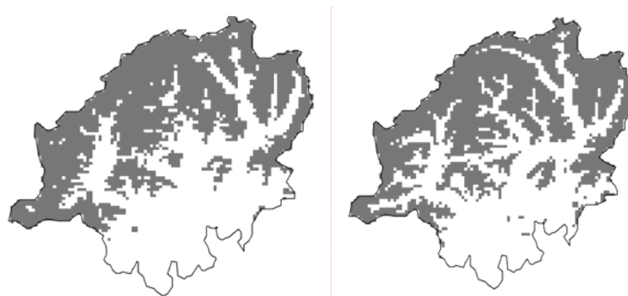
Fig. 8. Classified satellite image for 10 February 2002 at 14:30 (left) and simulated map (right) and the histogram of the number of pixels for the different type of coverage.
