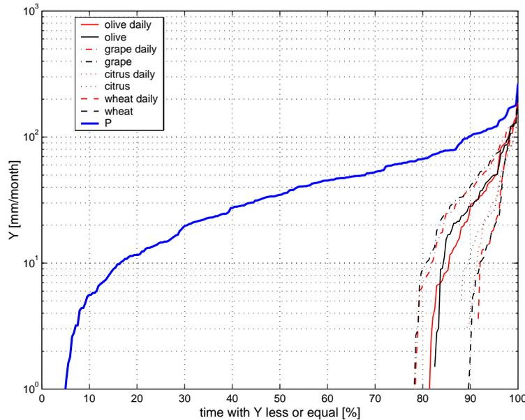
**Fig. B1** Comparison between daily and monthly estimation of mean annual water fluxes in response to variable soil moisture storage capacity,  $S_{bc} = S_{fc} - S_{wp}$ . Simulations were conducted with soil hydraulic parameter in the typical ranges of the silty-loam. Red marks refer to the daily model while black marks to the monthly one. Drainage response is in the lower part of the figure (decreasing patterns) and evapo-transpiration in the upper part.
