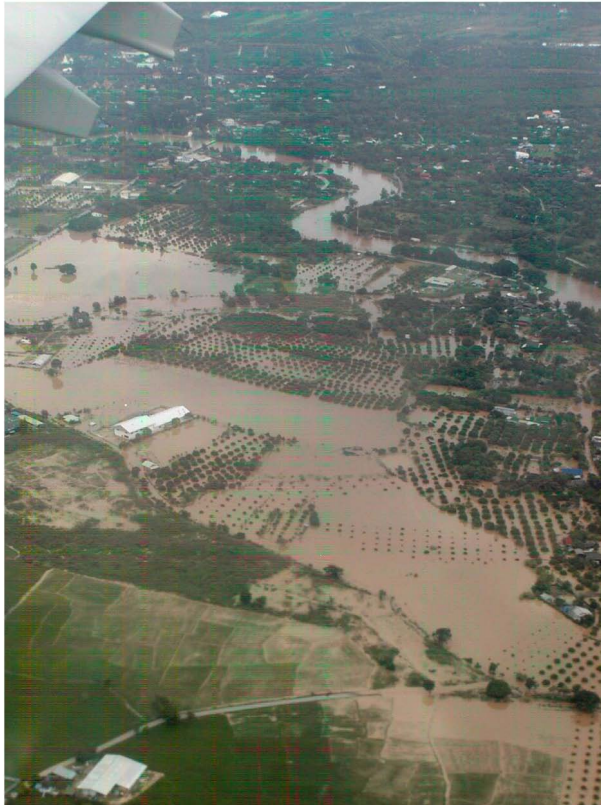
Fig. 7. Photo from airplane of the flooded area of the Ping River at peak flood flow 16:00, 29 September 2005. View is to the east toward the bridge at Ban Mae Kha. Tributary channel joins the river on the right (downriver) side of photo. Area of mapped sediment thickness (Fig. 5) extends from the white building (left center of photo) to the river.
