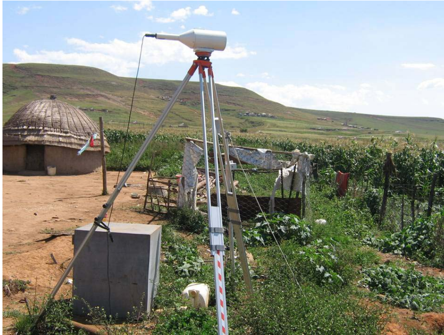
Fig. 10. The receiver of the Large Aperture Scintillometer in one of the homesteads in the Potshini catchment.
