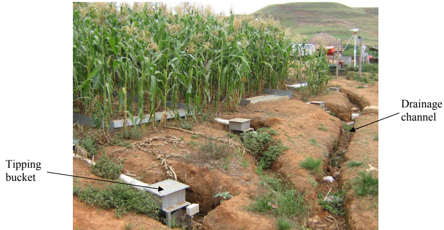
Fig. 6. A set of runoff plots under different treatments in a farmer managed trial.
