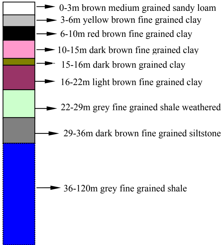
Fig. 8. Borehole log information including the lithology, grain size and colour for one of the deep observation groundwater wells in the Potshini catchment.
