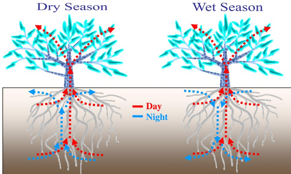
**Fig. 1.** Schematic description of the hydraulic redistribution.
