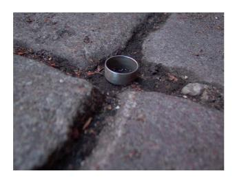
**Fig. 4.** Undisturbed sampling of seam material (0 to 1 cm) from a cobbled stone paved street using special 3.3 cm<sup>3</sup> cylinders in an old residential area at the site Pfluegerstrasse, Berlin.
