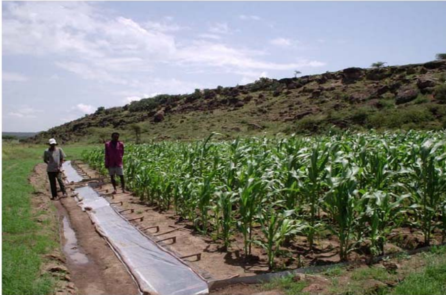
Fig. 5. Surface runoff collecting trough covered with hanging plastic sheets to prevent direct precipitation.
