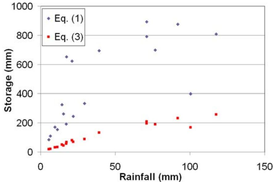
**Fig. 4.** Graph of total rainfall  $P$  versus total watershed storage  $S$ , at each storm event. Equation (1) takes into account the observed data for the determination of initial abstraction, while in Eq. (3) the initial abstraction is calculated from the SCS empirical equation.
