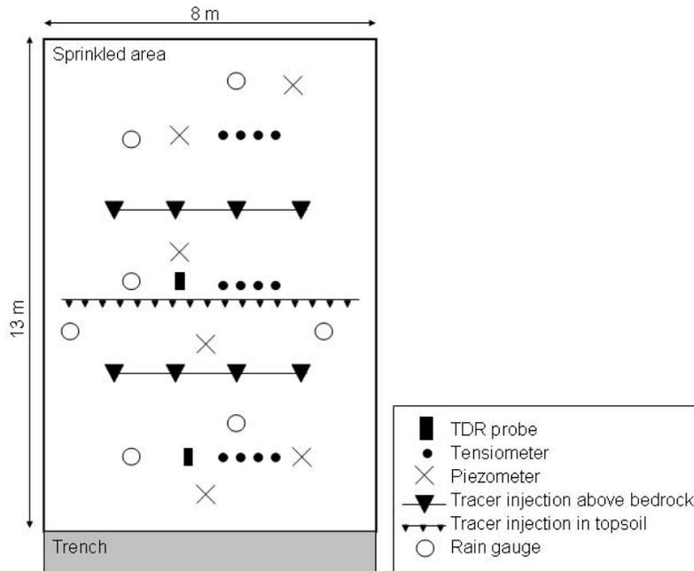
**Fig. 1.** Experimental set-up during the sprinkling experiments in a view from above. Installation depths of the probes and tracer injection varied at different experimental slopes according to soil depth.
