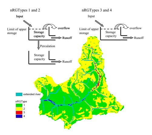
**Fig. 2.** Conceptualization of reservoirs of the different units of runoff generation types with extended river network.
