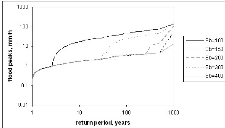
Fig. 8. Flood frequency curves generated by Model 4 using \eta=0.5 and various S_b .
