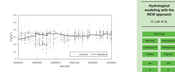
**Fig. 11.** Comparison of 60 cm depth averaged measured surface soil moisture content with saturation degree in the unsaturated zone,  $s^{u}$ , simulated by CREW.
