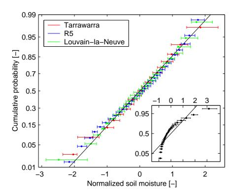
**Fig. 3.** Normal probability plot of the normalized spatial soil moisture fields. Dots indicate the median value, error bars indicate 25% and 75% percentiles of time variability. The inset shows the same procedure applied to randomly generated fields from a log normal distribution, with n=25 and k=60.
