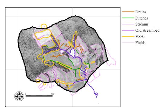
**Fig. 7.** Position of natural and artificial drainage features, and estimated frequently saturated hydrologic source area positions, as digitized from a 1-m resolution DOQQ.
