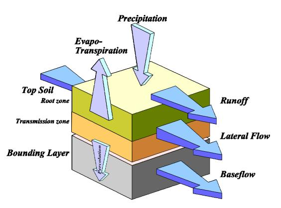
Fig. 1. Schematic representation of the water balance components over one cell.
