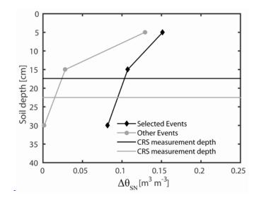
**Fig. 7:** Change in soil moisture ( $\Delta \theta_{S\lambda}$ ) at depths of 5, 15 and 30 cm at the JER for the five large events ('Selected Events') and the remaining ('Other Events') cases. Horizontal lines are the CRS measurement depths averaged over the corresponding cases (black is Selected Events, gray is Other Events).
