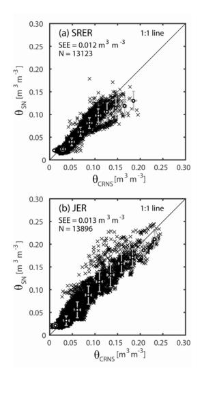
**Fig. 5:** Scatterplots of the spatially-averaged, hourly soil moisture  $(m^3/m^3)$  from <u>CRSCRNS</u> 7 method  $(\theta_{CRS}\theta_{CRNS})$  and distributed sensor network  $(\theta_{SN})$  at (a) SRER and (b) JER. The SEE and 8 the number of hourly samples (N) are shown for each site. Bin averages and ±1 standard
