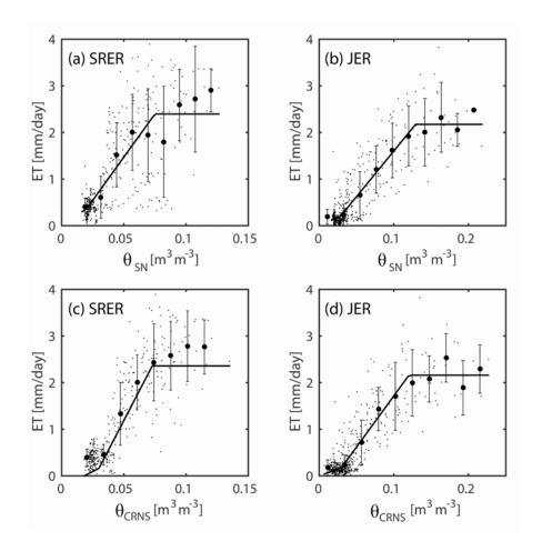
Fig. 10: Evapotranspiration relation with the spatially-averaged distributed sensor network ( $\theta_{SN}$ , top) and the <u>CRSCRNS</u> method ( $\theta_{CRS}\theta_{CRNS}$ , bottom) for (a, c) SRER and (b, d) JER. Bin averages and  $\pm 1$  standard deviation are shown (circles and error bars) for bin widths of 0.015  $m^3/m^3$  at SRER and 0.025  $m^3/m^3$  at JER. Regressions for the relations of ET with  $\langle \theta \rangle$  are valid for the entire dataset.
