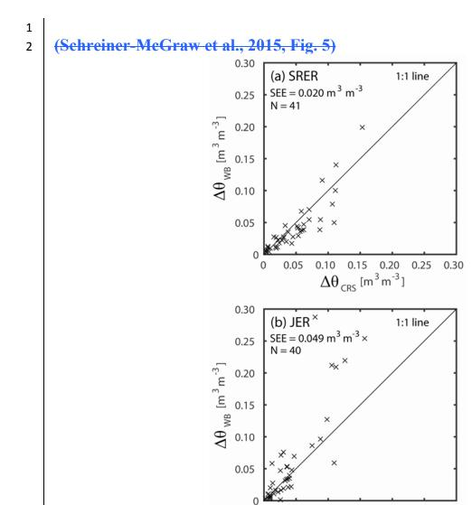
**Fig. 6:** Scatterplots of the spatially-averaged change in soil moisture (m<sup>3</sup>/m<sup>3</sup>) derived from CRS
