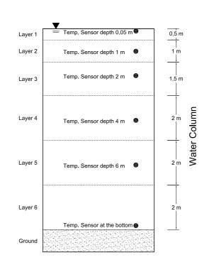
Fig. 1. Layers thickness and temperature sensors
