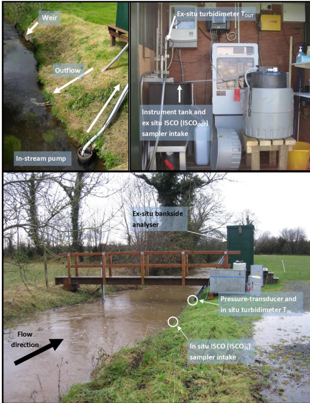
Figure C: Picture of in situ and ex situ suspended sediment and discharge instrumentation at Grassland B.
