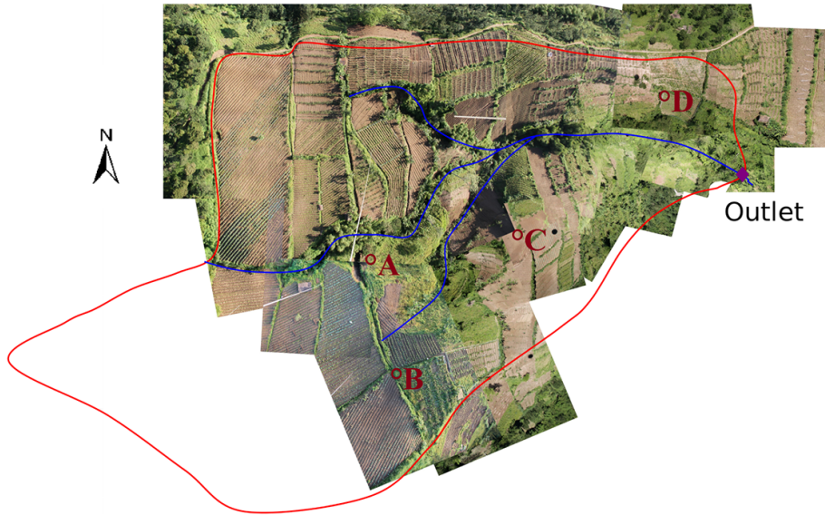
Figure 2. Assembly of aerial photographs. The basin boundaries are in red and the main hydrography in blue. Runoff was observed on the A, B, C and D locations.
