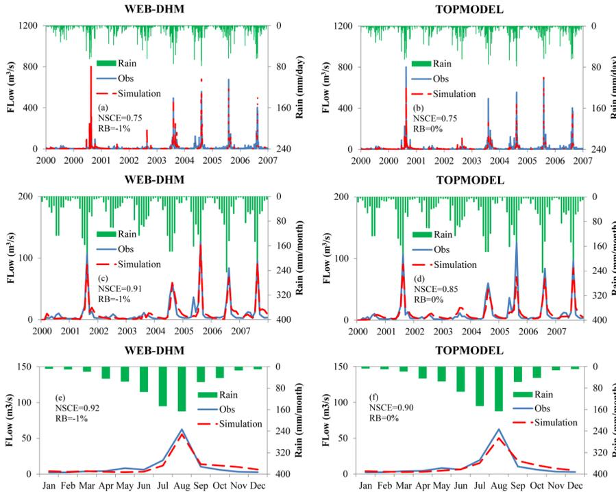
Figure 3. Observed and simulated flow using WEB-DHM and TOPMODEL from 2000 to 2007.
