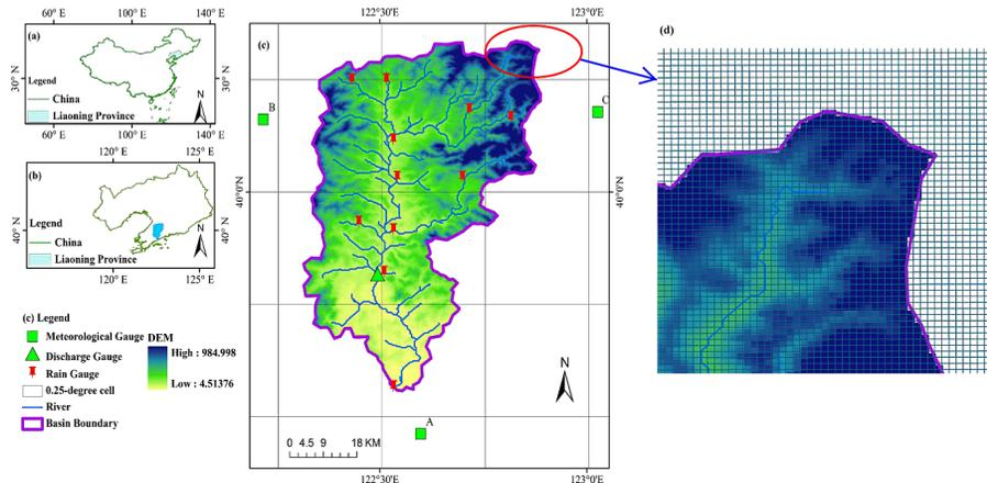
**Figure 1.** Biliu basin: **(a)** the location of Liaoning province within China; **(b)** the location of Biliu basin within Liaoning province; **(c)** the distributions of rain gauges, discharge gauge, automatic weather stations, digital elevation model, and diagrammatic 0.25° precipitation cells; and **(d)** diagrammatic description of downscaling the 0.25° precipitation cells to 300 m × 300 m cells, and retrieving the 300 m × 300 m cells located within the basin boundary.
