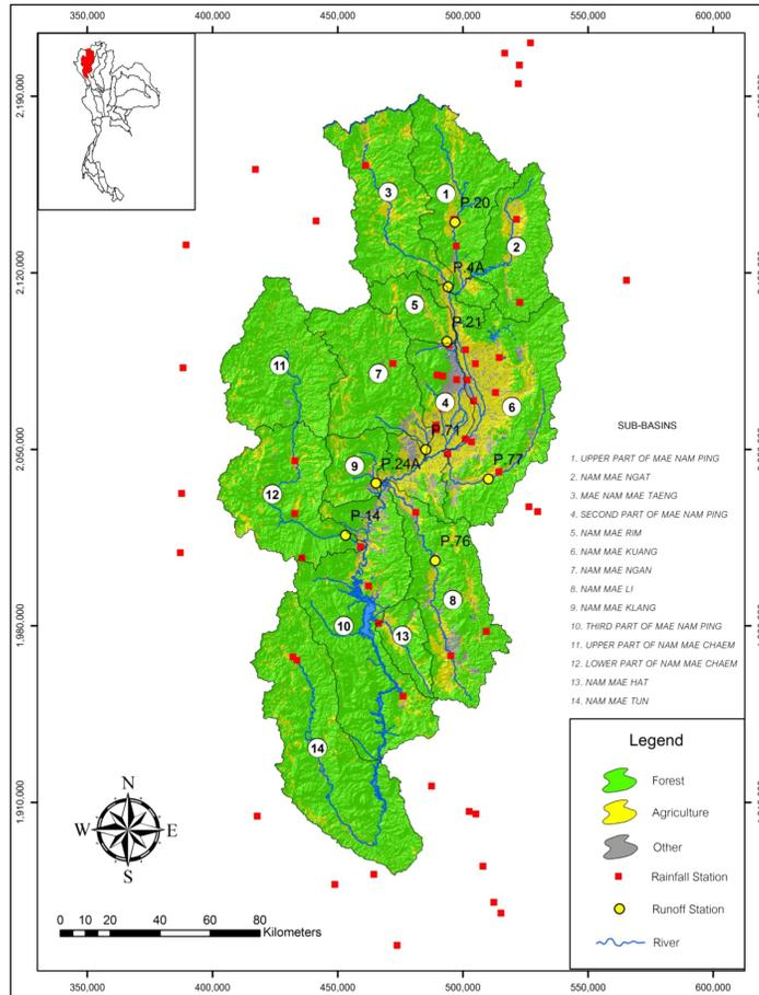
**Figure 2.** The Upper Ping River Basin (UPRB) and the locations of the rain-gauge and runoff stations. The numbers indicate the 14 sub-basins of the UPRB.
