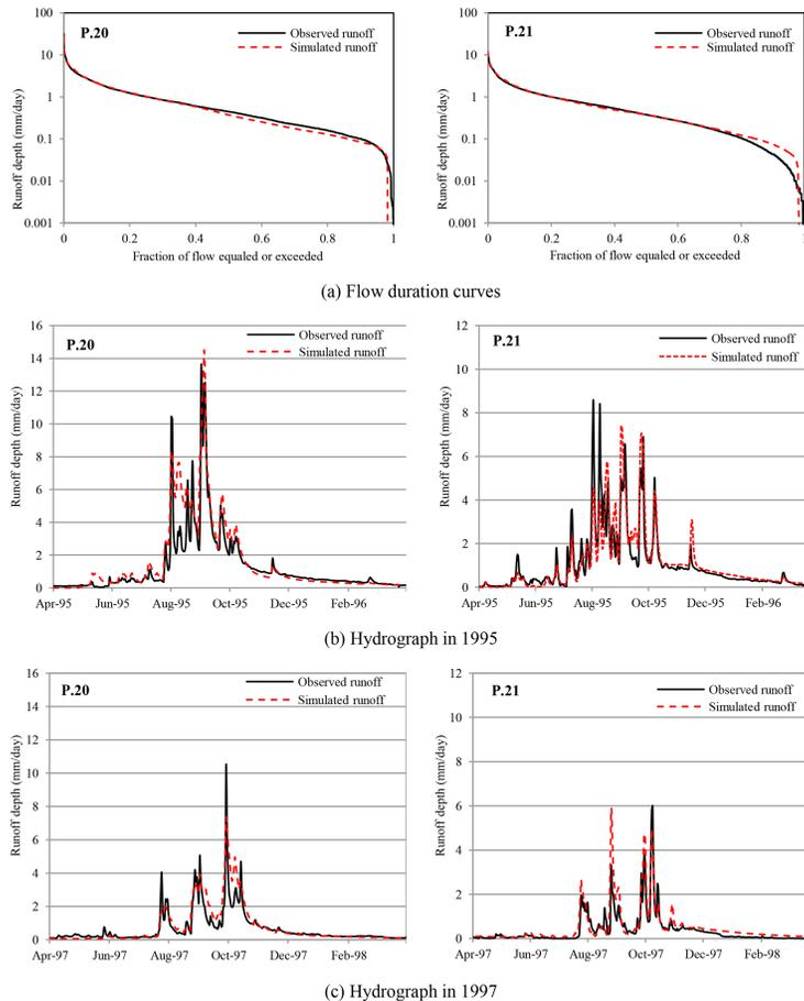
**Figure 5.** Examples of flow duration curves and simulated hydrographs using FLEX<sup>L</sup> at runoff stations P.20 and P.21.
