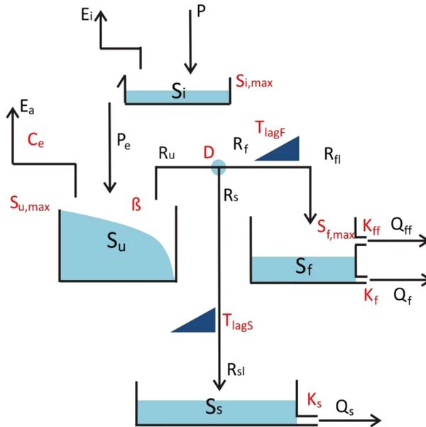
**Figure 1.** Model structure of the FLEX<sup>+</sup>.
