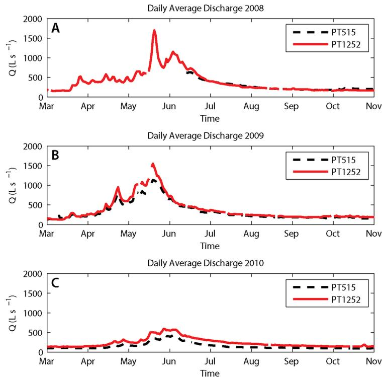
**Figure 2.** Daily average discharge estimated from continuous pressure transducer records spanning 2008–2010 (a–c). The black dashed line represents upstream, inflow conditions at PT515 and the red solid line represents downstream, outflow conditions at PT1252.
