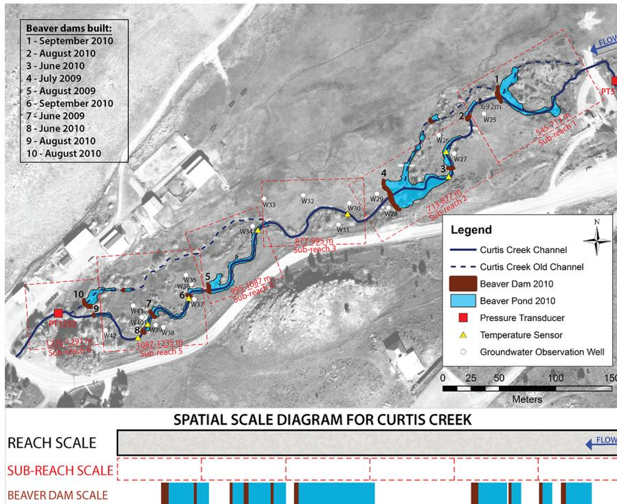
**Figure 1.** Aerial image from 2006 and beaver dams constructed between 2009 and 2010. The main beaver dams are numbered from 1 to 10 from upstream to downstream and the time of dam construction is noted in the table. The study reach was further divided into 6 sub-reaches. The spatial scales investigated are illustrated below the map. The most downstream beaver dam and beaver pond are located in the old channel but overlap in the Beaver Dam Scale schematic in this figure.
