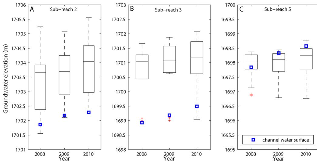
**Figure 8.** Groundwater elevation throughout the study reach grouped by individual sub-reaches and water surface elevation in the channel for each sub-reach. The water surface elevation in the channel represents the average yearly value for each sub-reach. There is a gradual increase in groundwater elevation and channel water surface elevation in all sub-reaches over the years.
