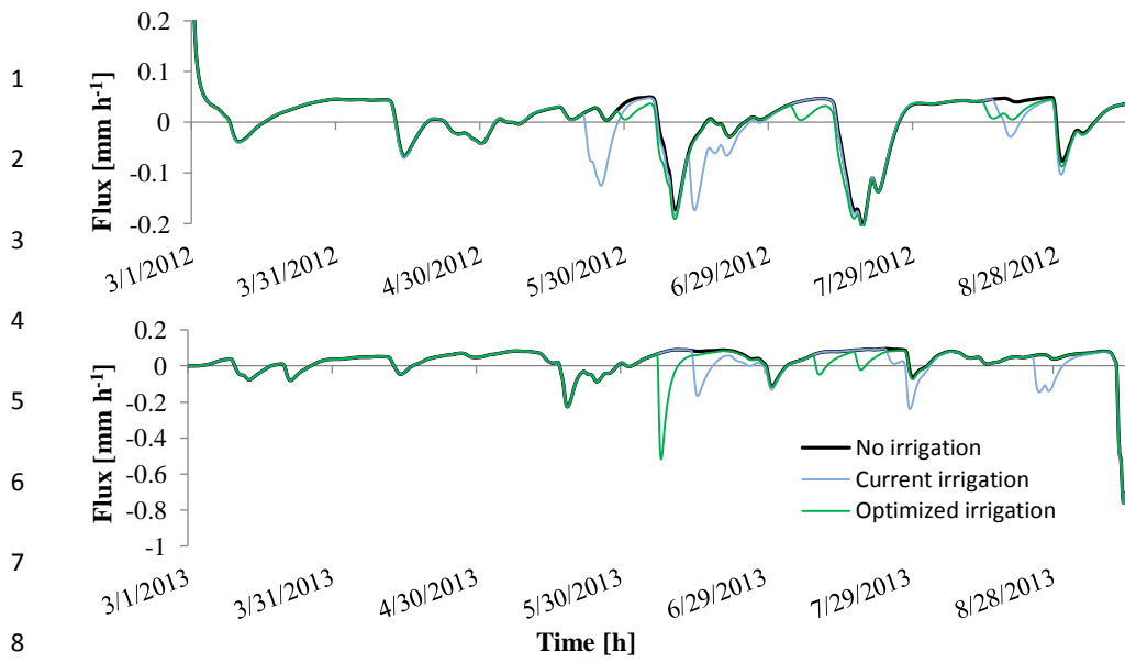
9 Figure 8. Actual flux of farmer's conventional irrigation (current irrigation), without irrigation 10 and optimized irrigation scheme (guided irrigation) for 2012 and 2013.
