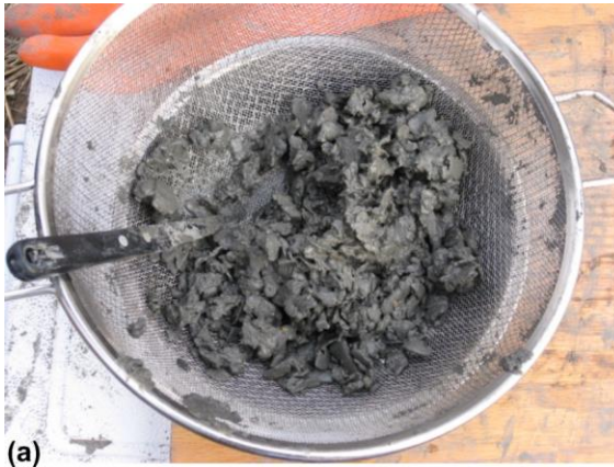
Figure 3. Evaluation of core cuttings as an alternative sample source for DVE-LS: (a) sieved chip samples after washing, and (b) wiped chip samples (typically 25 × 15 mm) prior to placement in Ziploc™ bags.
