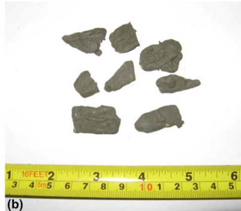
Figure 3. Evaluation of core cuttings as an alternative sample source for DVE-LS: (a) sieved chip samples after washing, and (b) wiped chip samples (typically 25 × 15 mm) prior to placement in Ziploc™ bags.
