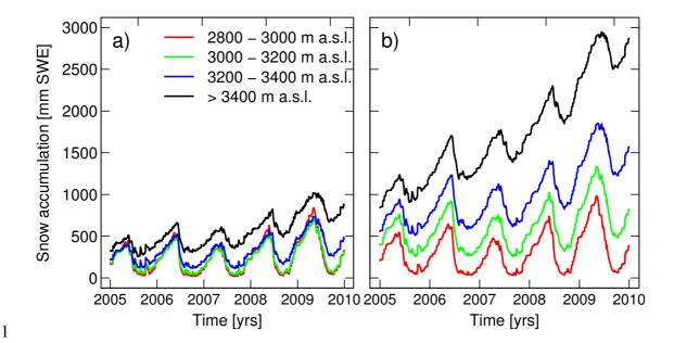
Figure 10. Behaviour of snow accumulation and melt of model A (a) and B (b) in the upper elevations. Note that model results are shown from 2005 to 2010 without the warm-up period for clarity reasons. Therefore snow depth does not start at zero in the figure while it does at the beginning of the modelling.
