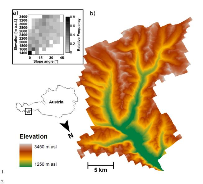
Figure 6. Elevation levels of the Ötztal using a 1x1 km grid (b). Frequency distribution of slope angles derived from 1x1 km grid are shown (a). Slopes in general are steeper in the summit regions than in the valleys. Note that instead of the average slope of a grid cell only steepest vertical gradients are plotted.
