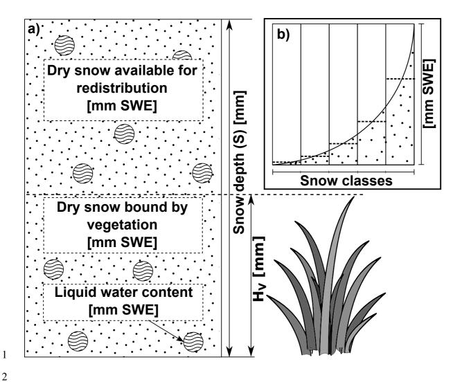
Figure 2. Schematic view of the snow cover in COSERO. a) Composition of one snow class. Vegetation or surface roughness defines the threshold value (H<sub>V</sub>) to hold back an amount of snow. b) View of one grid cell including five snow classes each of which is composed in the way shown in a). Snowfall is distributed log-normally throughout the classes (dashed lines in b)). Note that snow depth S is given in mm while all other parameters regarding snow are given in mm SWE.
