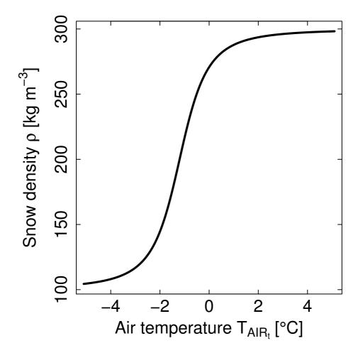
Figure 3. Estimation of the density of snow using Eqs. (8) and (9). Minimum and maximum densities of fresh snow are 100 and 300 kg m<sup>-3</sup>, respectively.
