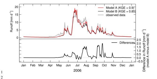
Figure 7. Specific runoff at the outlet at Huben is modelled with (model A) and without (model B) using the snow redistribution routine.
