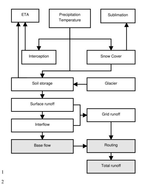
3 Figure 1. Flow chart of the conceptual model COSERO. White parts represent distributed
