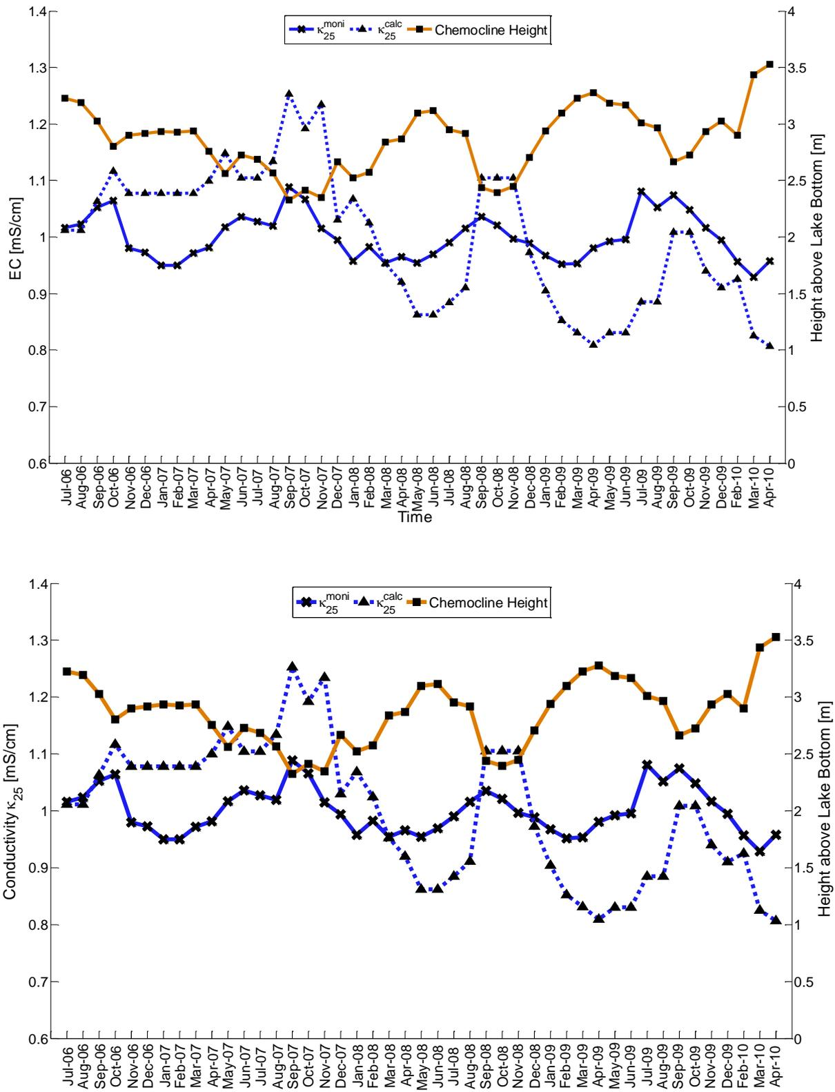
**Figure 9:** Comparison of time series of measured and calculated average electrical conductivity ( $\kappa_{25}$ ) in the monimolimnion.
