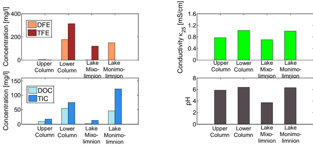
**Figure 6:** Iron species content (DFE and TFE), electrical conductivity, carbon species content (DOC and TIC) and pH-value of samples from different water layers in [Lake Waldsee](#) and the water column
