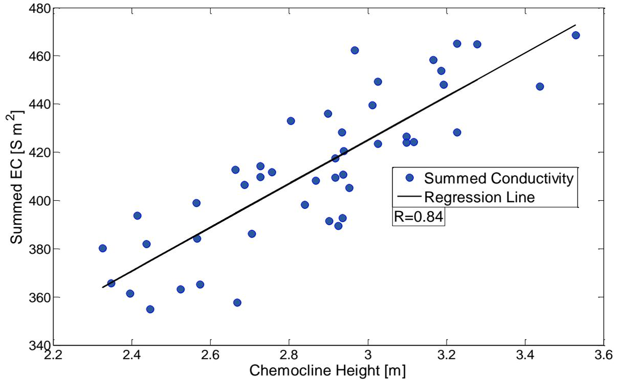
**Figure 8:** Correlation between summed conductivity and chemocline height. A linear regression results in a correlation coefficient of 0.84.
