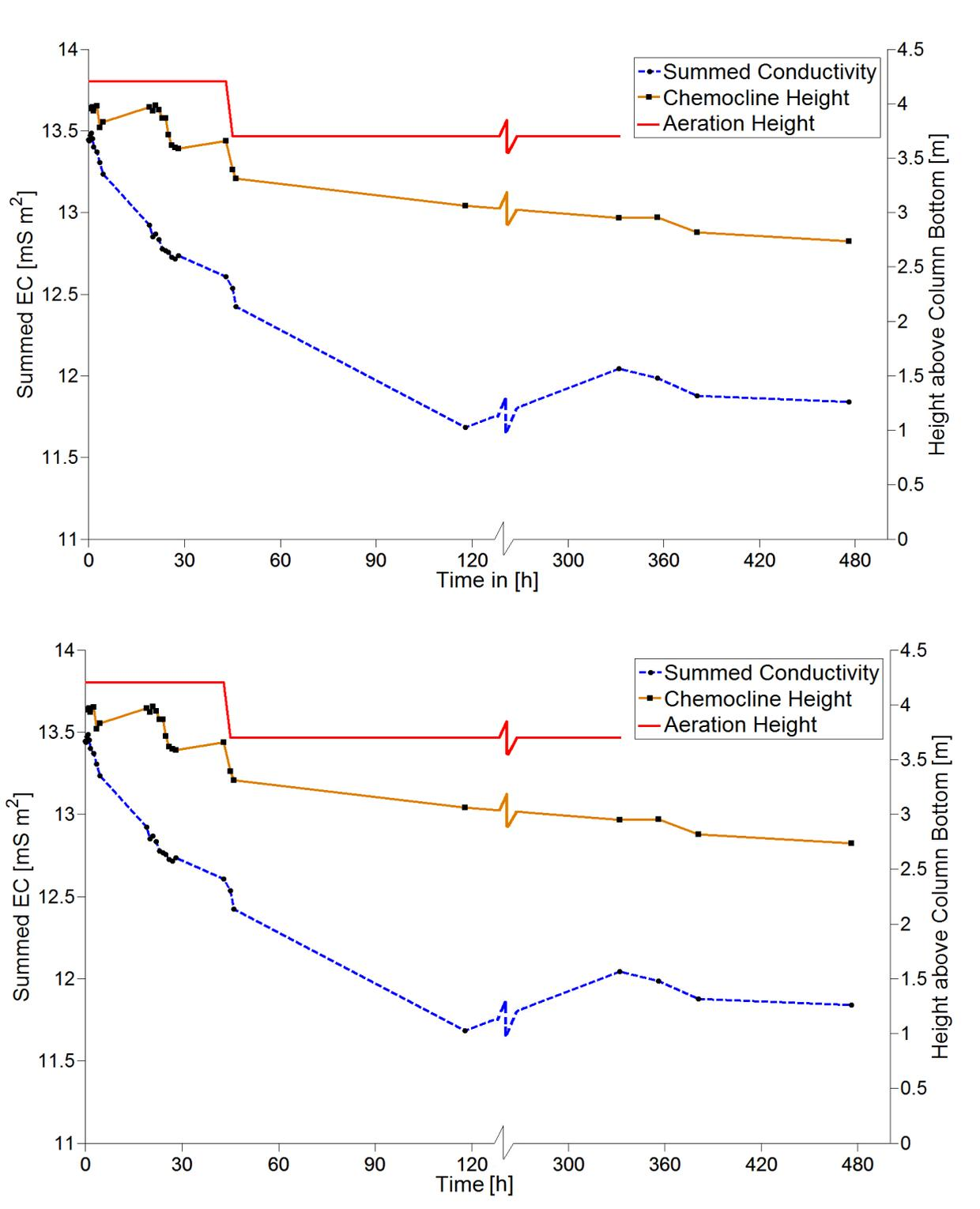
**Figure 4:** Temporal dynamics of chemocline height and summed conductivity (EC) during the column experiment. The scale breakage indicates the end of the hourly range sampling period of the experiment.
