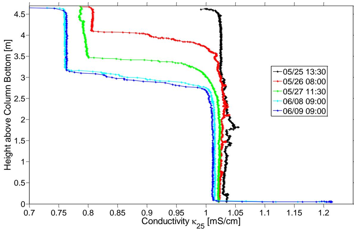
**Figure 5:** Selected conductivity ( $\kappa_{25}$ ) profiles at different time steps of the lab experiment. The earliest profile shows the initial condition in the water column followed by two profiles during active aeration at a depth of 0.5 m and 1 m, respectively. Last two profiles show the conductivity distribution in the column a certain time after cessation of aeration. profiles in the lab experiment
