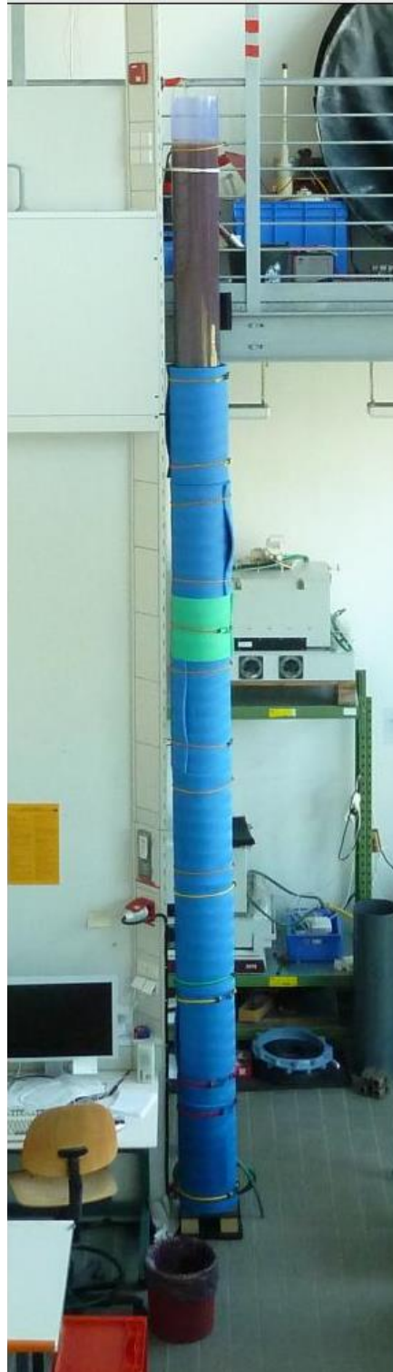
Figure 3: Initial conditions of the water column experiment: brownish monimolimnion water in a PVC pipe, thermally insulated by PE mattresses. Uppermost mattresses were removed for the purpose of this photograph.
