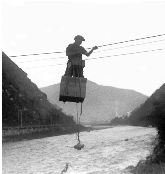
Figure 2. Stream flow measurements at the gauge station “Borgo a Mozzano” ( 43^{\circ}59'30.73'' N; 10^{\circ}33'10.04'' E) in the River Serchio (Italy), probably taken in the 1920s or 1930s. The observer is placed in a box suspended on cable that moved along the cross section from which manages an old device to measure the stream flow velocity (Photo courtesy of Regione Toscana – Genio Civile di Bacino Toscana Nord e Servizio Idrologico Regionale).
